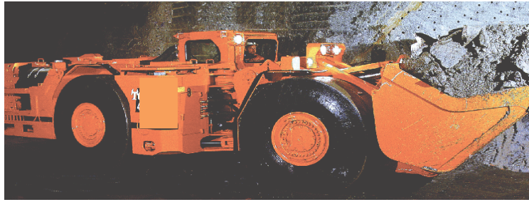
Figure 1. Example LHD vehicle used in underground mining The vehicle shown is approximately 2.7 m wide, 2.5 m high, 10.5 m long with a 5.4 m 3 bucket
